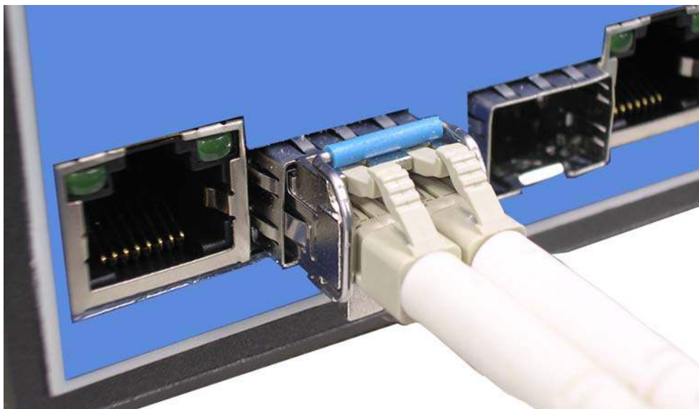
Figure 2.10: LC connector to the transceiver
