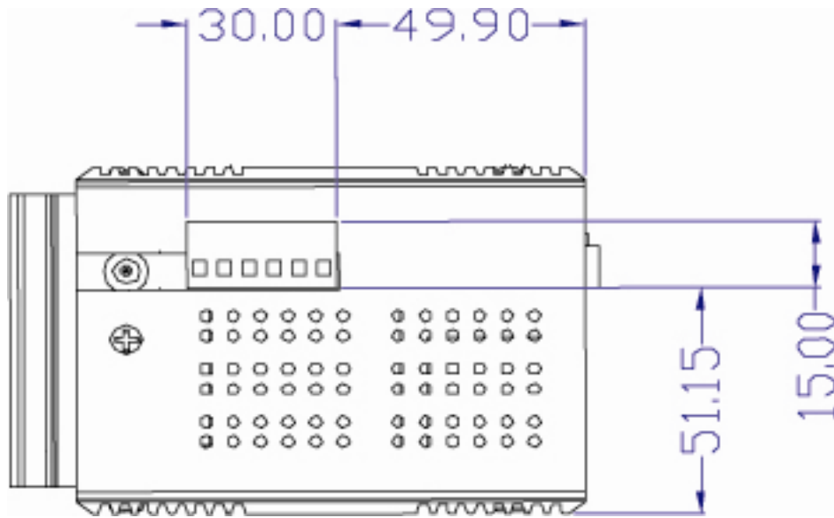
Figure 2.4: Top View of EKI-7626C/7626CI
