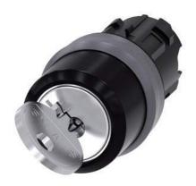
RONIS key-operated switch, 22 mm, round, plastic with metal front ring, lock number SB30, with 2 keys, 2 switch positions O<I, momentary contact type, Actuating angle 45°, 10:30h/12h, key removal O, possible special locks: SB31, 421, 455, with laser labeling, inscription or symbol Customerspecific selection with SIRIUS ACT configurator (CIN)
