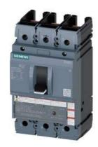
circuit breaker 3VA5 UL frame 250 breaking capacity class M 35kA @ 480V 3-pole, line protection TM230, FTAM, In=90A overload protection Ir=90A fixed short-circuit protection Ii=5...10 x In UL 489 SB (naval), 50 °C without connection
