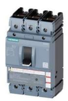
circuit breaker 3VA5 UL frame 250 breaking capacity class M 35kA @ 480 V 3-pole, line protection TM230, FTAM, In=175A overload protection Ir=175A fixed short-circuit protection Ii=5...10 x In UL489 SB (naval), 50 deg. cel. cable connection on both sides
