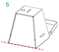
With the case orintated like the image above, fold the side closest to you. This will leave the correct side open for the next step.
