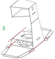
Fold marked lines and push the second tab through the other slot.
