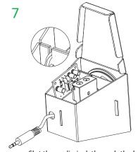
Slot the audio jack through the hole, insert electronics into the designated compartments & ensure wires are sat in the notches provided.
