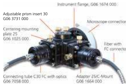
Mounting example for the instrument flange
