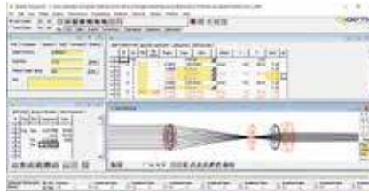
Simulation of the beam path of a basic alignment telescope with Qioptiq WinLens™
