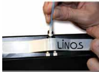
Pressing down and repositioning a mirror on the fixed mirror mount
