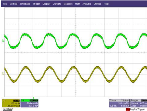
Figure 17 – 90 VAC, Full Load. Upper: I_{IN} , 0.2 A / div. Lower: V_{IN} , 200 V, 10 ms / div.
