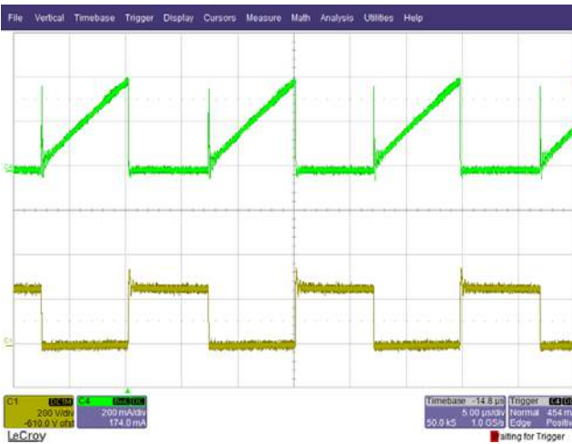
Figure 19 – 90 VAC, Full Load. Upper: I_{DRAIN} , 0.2 A / div. Lower: V_{DRAIN} , 200 V, 5 \mu s / div.
