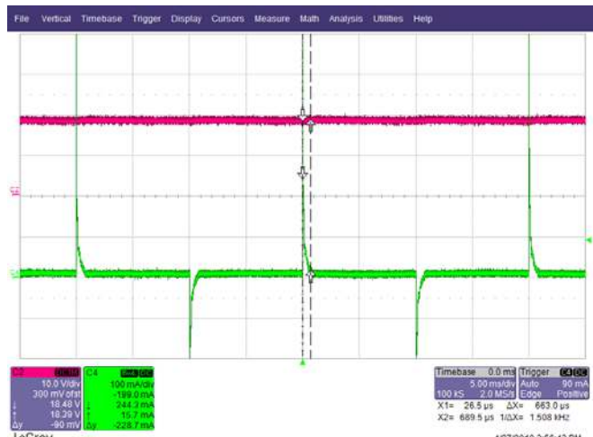
Figure 37 – 230 VAC, 12° Phase. Upper: V_{OUT} , 10 V / div. Lower: I_{IN} , 0.1 A / div., 5 ms / div.
