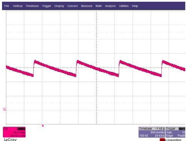
Figure 28 – Output Voltage: 230 VAC. V_{OUT} , 10 V / div., 500 ms / div.
