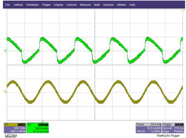
Figure 18 – 265 VAC, Full Load. Upper: I_{IN} , 0.1 A / div. Lower: V_{IN} , 500 V / div., 10 ms / div.
