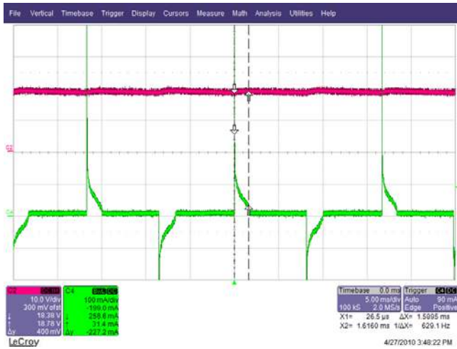
Figure 32 – 115 VAC, 35° Phase. Upper: V_{OUT} , 10 V / div. Lower: I_{IN} , 0.1 A / div., 5 ms / div.
