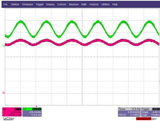
Figure 21 – 90 VAC, Full Load. Upper: I_{RIPPLE} , 0.2 A / div. Lower: V_{OUTPUT} 5 V, 5 ms / div.
