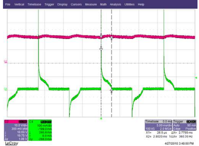
Figure 31 – 115 VAC, 60° Phase. Upper: V_{OUT} , 10 V / div. Lower: I_{IN} , 0.1 A / div., 5 ms / div.
