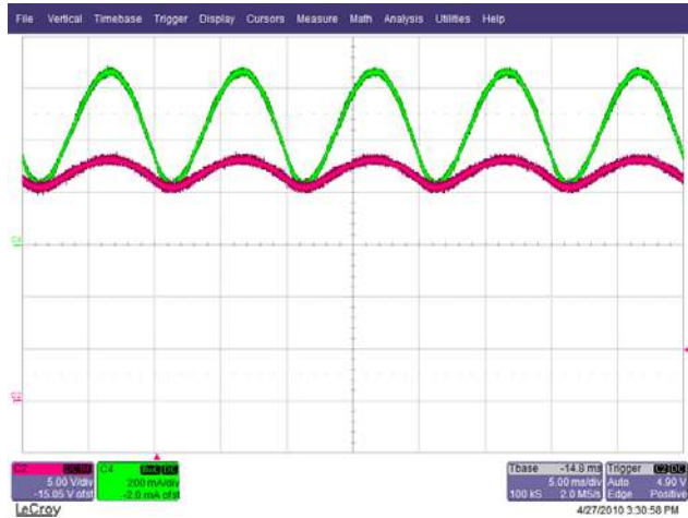
Figure 22 – 265 VAC, Full Load. Upper: I_{RIPPLE} , 0.2 A / div. Lower: V_{OUTPUT} 5 V, 5 ms / div.
