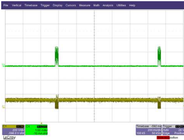
Figure 25 – 90 VAC, Full Load. Upper: I_{OUTPUT} , 1 A / div. Lower: V_{DRAIN} , 200 V, 200 ns / div.
