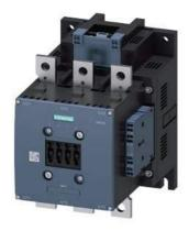
power contactor, AC-3 300 A, 160 kW / 400 V, AC (50-60 Hz) / DC operation 96-127 V AC/DC auxiliary contacts 2 NO + 2 NC 3-pole, frame size S10 busbar connections drive: electronic with PLC interface 24 V DC spring-loaded terminal
