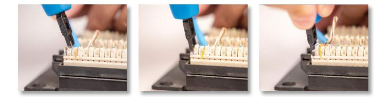
Designed as an economical option for seating and trimming wire in 110 type punchdown blocks, th PD-110 is perfect for small do-it-yourself jobs on 110-terminal blocks. This non-impact punchdown tool features the following:
