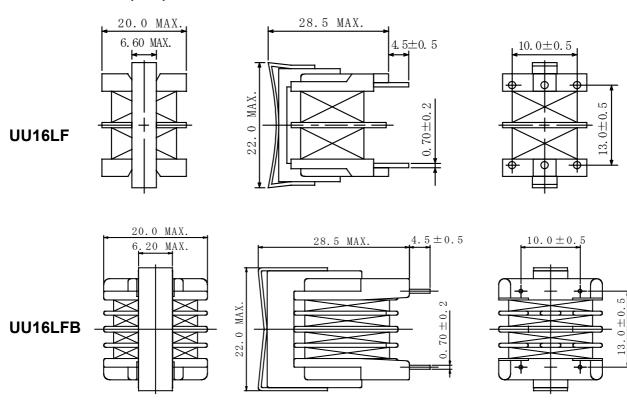
\* Dimension does not include solder used on coil.
