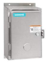
Non-reversing NEMA contactor, Size 1, 4 power poles, Contactor amp rating 27A, 3 wire (NO aux included), 110V 50Hz / 120V 60Hz coil, Non-combination type, Encl NEMA type 4X 304 S-Steel, Water/dust tight noncorrosive, Standard width enclosure
