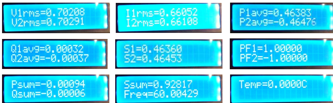
Figure 9. Standalone Power Meter Measurements
