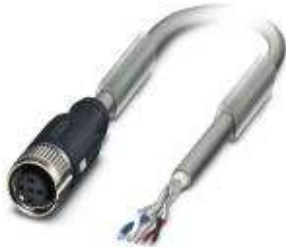
Bus system cable, CANopen®, 5-position, PUR halogen-free, Gray RAL 7001, Free cable end, on Socket straight M12-SPEEDCON, A-coded, Cable length: 10 m
