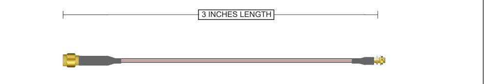
Connector A 132114RP SMA Plug Straight Brass Gold + Heatshrink 50 Ohm RG-316 Continuity/Hi-Pot Connector B 262121 MMCX Jack Straight Bulkhead - Rear Mount Brass Gold + Heatshrink
