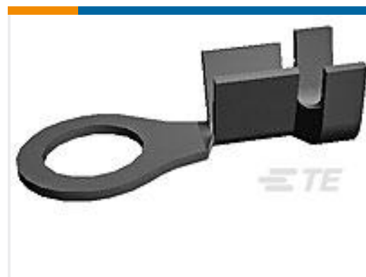
TE Part #40661 RING 190(4.82 MM) TERMINAL 18-14 AWG BR
