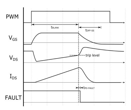
Over-Current Protection Timing Diagram
