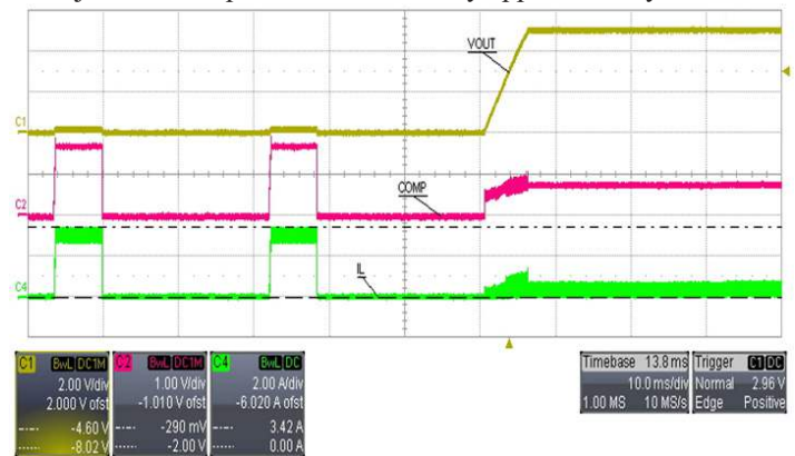
Figure 10: Hiccup Mode and Recovery (to 5 V at 0.5 A, for A8591, shown)
