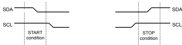
Figure 21-3. START and STOP Conditions
