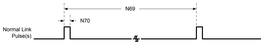
Figure 30-38. 10Base-TX Normal Link Pulse Timing
