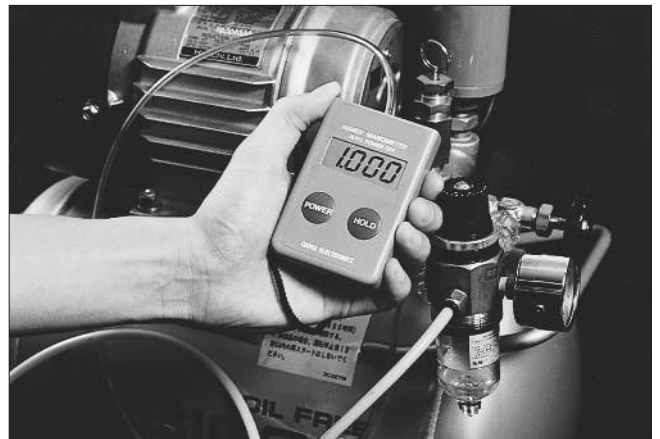
▲ Measurement of source pressure from a compressor.
