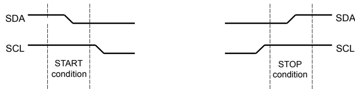
Figure 16-3. START and STOP Conditions
