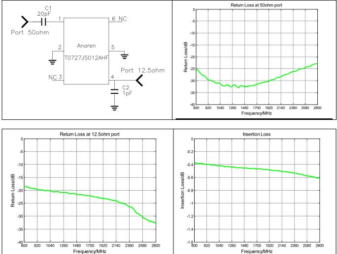
DC connectivity of T0727J5012AHF with pin assignments is shown below. It is noted here that pin3 and pin6 are NC pins without any internal connections, while pin1, pin4, pin 2 and pin 5 are DC connected internally together. To have T0727J5012AHF function properly, pin 2 and pin 5 are required to be grounded by the mounting footprint.
