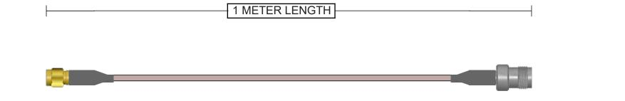
Connector A 132195 SMA Plug Straight Brass Gold + Heatshrink 50 Ohm RG-142 Continuity/Hi-Pot Connector B 031-2380 TNC Jack Straight Brass Nickel + Heatshrink
