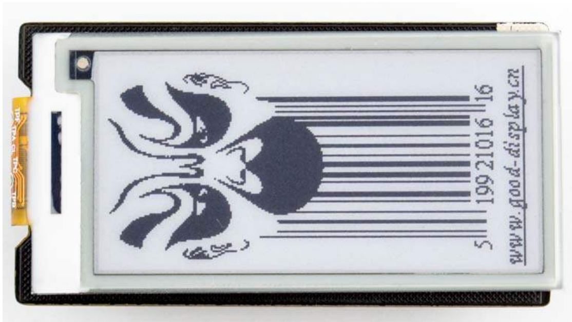
FireBeetle Covers-ePaper Black&White Display Module(SPI)
