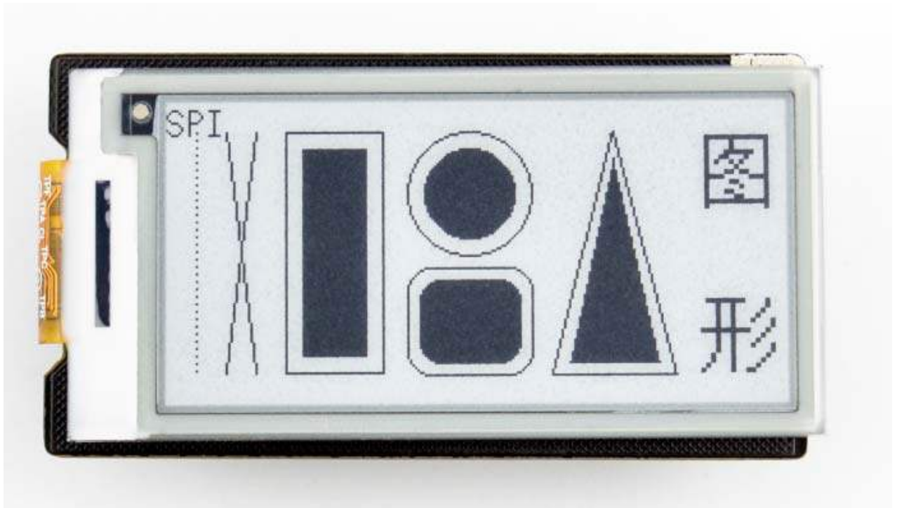
FireBeetle Covers-ePaper Black&White Display Module(SPI)
