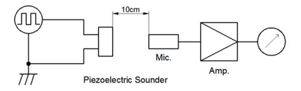
MIC: ND10 Sound Meter or equivalent Signal Generator: DF1641D or equivalent
