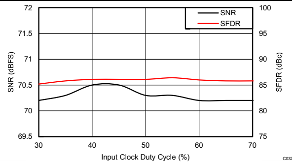
Figure 98. Performance vs Clock Duty Cycle (150 MHz)
