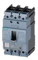
circuit breaker 3VA5 UL frame 125 breaking capacity class M 35kA @ 480 V 3-pole, line protection TM230, FTAM, In=110A overload protection Ir=110A fixed short-circuit protection Ii=5...10 x In cable connection on both sides
