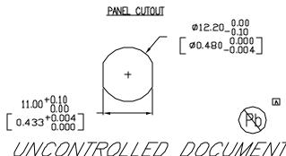
\*UNLESS DTHERWISE SPECIFIED TOLERANCES PER DECINAL PRECISION ARE: X=±1 (±0.039), XXX=±0.5 (±0.020), XXX=±0.127 (±0.005). LEAD SIZE=±0.05 (±0.002), LEAD LENGTH=±0.75 (±0.010). MN= +DECINAL PRECISION MAX.= +0.00 (±0.005). LEAD SIZE=±0.05 (±0.002), LEAD LENGTH=±0.75 (±0.010). MN=+DECINAL PRECISION MAX.= +0.00 (±0.005).
