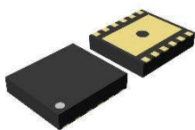
DFN(PL)2730-12 2.7 mm x 3.0 mm x 0.6 mm
