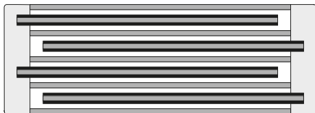
Extended double side metallized carrier film design
