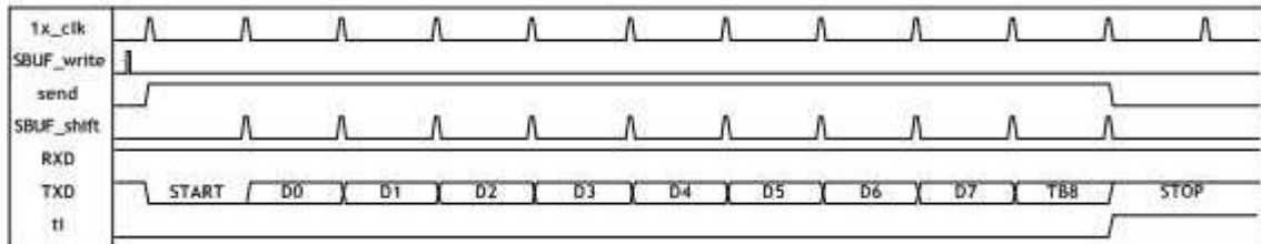
Figure 6.10 Timing Diagram for UART Transmission Mode3
