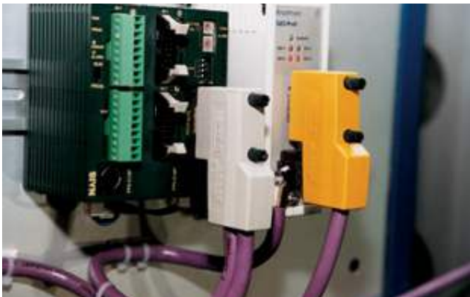
Pure nodes and termination versions. Color differentiation between node and termination within the bus
