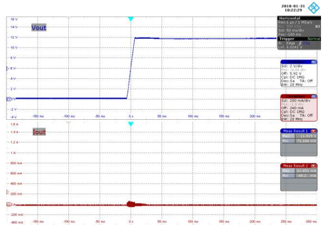
Figure 57 – 115 VAC 60 Hz, No-Load Start-up. Upper: V_{OUT} , 2 V / div., 50 ms / div. Lower: I_{OUT} , 200 mA / div., 50 ms / div.
