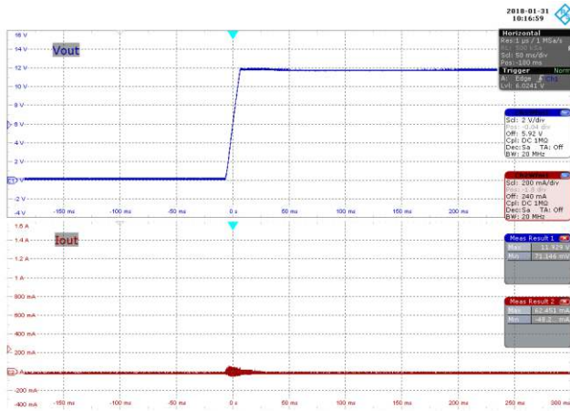
Figure 48 – 90 VAC 60 Hz, No-Load Start-up. Upper: V_{OUT} , 2 V / div., 50 ms / div. Lower: I_{OUT} , 200 mA / div., 50 ms / div.
