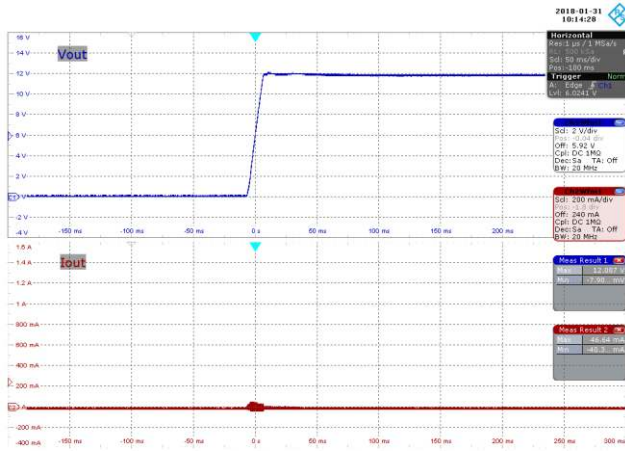
Figure 48 – 90 VAC 60 Hz, No-Load Start-up. Upper: V_{OUT} , 2 V / div., 50 ms / div. Lower: I_{OUT} , 200 mA / div., 50 ms / div.
