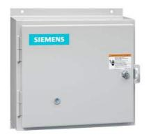
Non-reversing motor starter, Size 1, Three phase full voltage, Solid-state overload relay, OLRelay amp range 3-12a, 550/575 600 50/60HZ coil, Non-combination type, Enclosure type 12, Dust/drip proof for indoors, Standard width enclosure
