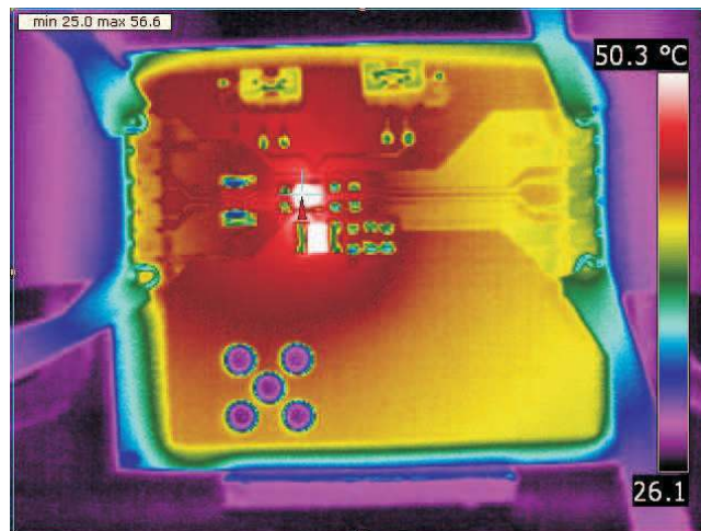
Figure 16. TPS62060EVM Thermal Performance
