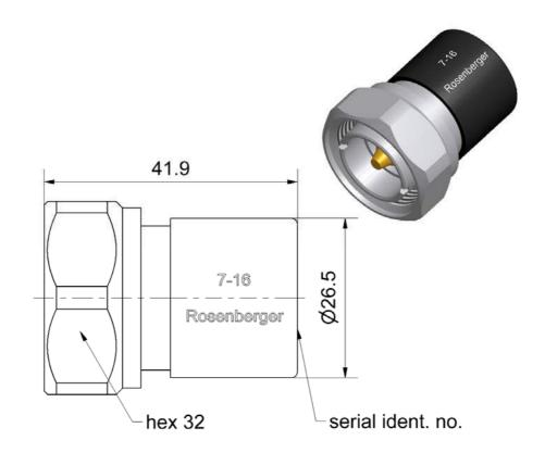
All dimensions are in mm; tolerances according to ISO 2768 m-H
