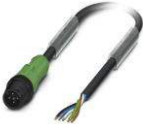
Sensor/Actuator cable, 5-position, PUR halogen-free, Black-gray RAL 7021, Plug straight M12, A-coded, on Free cable end, Cable length: 5 m, with plastic knurl
