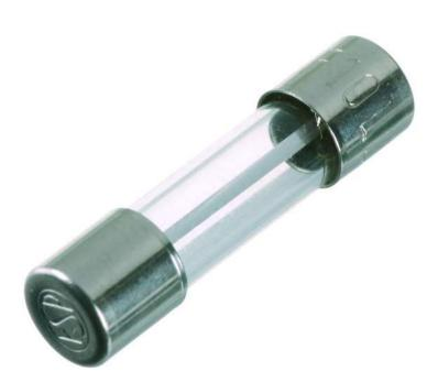
Fuse, Dimensions: 5x20 mm, Trigger characteristic: Fast-acting (F); Rated voltage: 250 V, Rated current: 1.6 A
