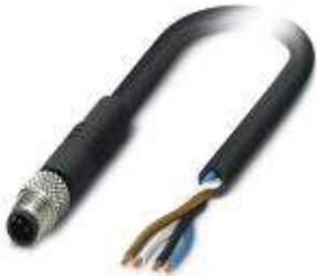
Sensor/Actuator cable, 4-position, PUR, Black RAL 9005, Plug straight M5, A-coded, on Free cable end, Cable length: 3 m
