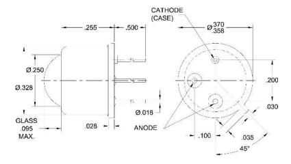
All surfaces are gold plated. Dimensions are nominal values in inches unless otherwise specified. Two Anode pins *must be* externally connected together.
