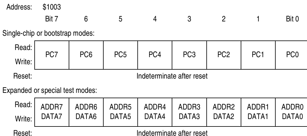
Figure 6-4. Port C Data Register (PORTC)
