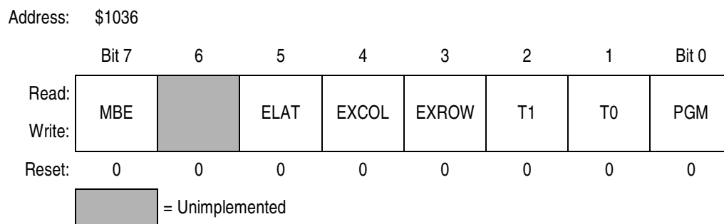
Figure 4-15. MC68HC711E20 EPROM Programming Control Register (EPROG)
