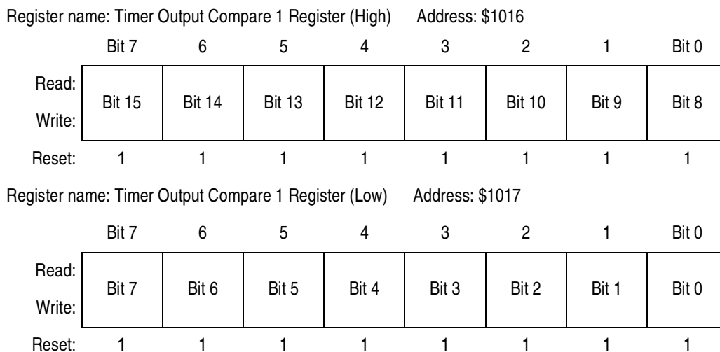
Figure 9-8. Timer Output Compare 1 Register Pair (TOC1)
