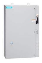
Non-reversing motor starter, Size 4, Three phase full voltage, Solid-state overload relay, OLR amp range 50-200A, 240V 50Hz / 277V 60Hz coil, Combination type, 200A fusible disconnect, 200A/600V fuse clip, Enclosure NEMA type 4/12, Water/dust tight for outdoors, Standard width enclosure
