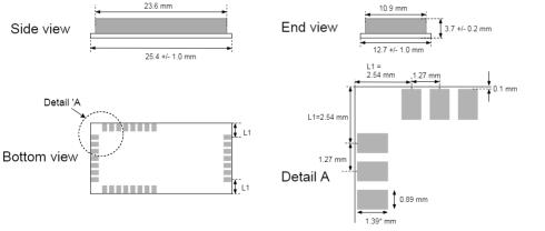
\*The pads might be slightly shorter than 1.39 mm due to PCB processing. The reduction will come from pad being pulled away from edge with up to 0.12 mm. This leaves a minimum pad lenght of 1.27 mm. The 0.1 mm distance to board edge is increase with the same number.
