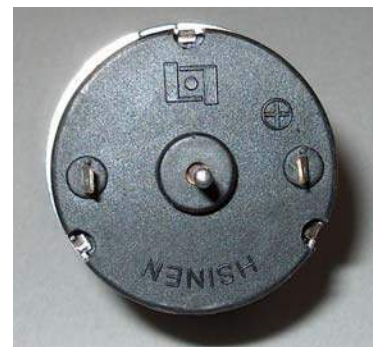
Back side of motor; note the ⊕ symbol to help match polarity.
