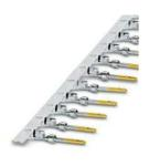
Crimp contact, Pin, rolled, Taped articles, number of pieces per reel: 500, contact diameter: 1 mm, crimp range: 0.22 mm $^2$  ... 0.56 mm $^2$ , Item is lead-free in accordance with RoHS II without Exemption 6c (Pb <0.1%)
