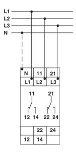
Phase failure: Output relay "R" drops out and yellow "REL" LED is OFF
