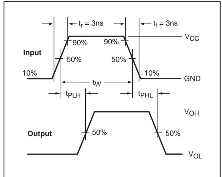
**Figure 3. AC Waveforms**
