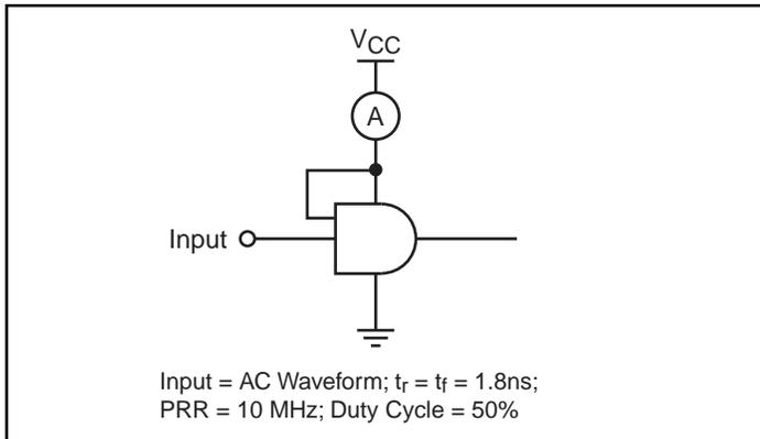
**Figure 2. I<sub>CCD</sub> Test Circuit**
