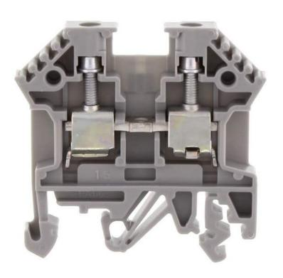
Feed-through terminal, Screw connection, Mounting type:Mounting rail TS 35/7.5 and TS 32, Rated cross-section: 4 mm², Width: 6 mm, Colour: Grey
