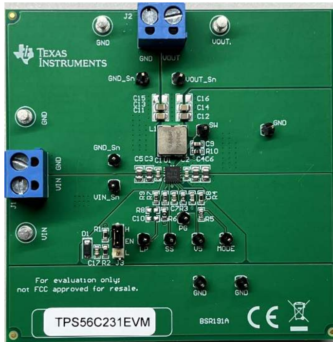
Figure 6-1. Top View of TPS56C231EVM
