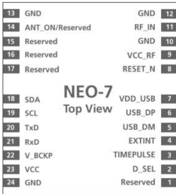
Figure 2: NEO-7 pin assignment
