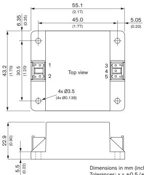
Dimensions in mm (inch) Tolerances: x.x  $\pm 0.5$  ( $\pm 0.02$ )
